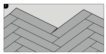
The boards need to be locked into one another, using the click lock system. To connect a new board you have to use a rubber hammer.
