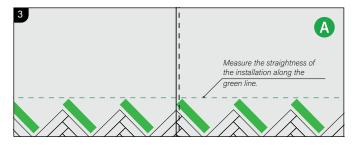
Install A-strips to connect all triangles. The joints between the A-strip and the triangle need to be checked very carefully. No protruding edge may be felt!
