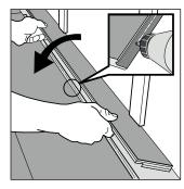
Remove the locking element according to the picture. Use an applicable glue to connect the strips. Press-place wedges between the glued strip and the wall.
