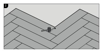
Use a rubber hammer and slightly knock at the click lock system to connect the short side. Start in the corner and work towards the end of the board.
