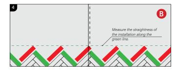
Now install B- strips and cut the most right piece to size.
